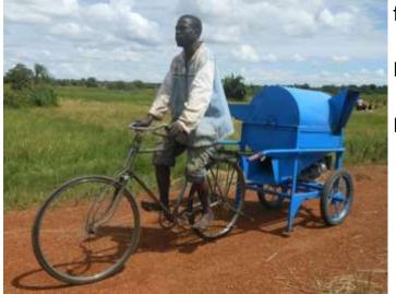
Weighs only 138 – 150kg compared to those other threshers weighing 350 – 1,000kg
